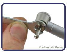
3. Tighten with the spanner. Do not overtighten.
