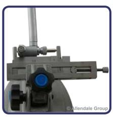
Slip gauges can be used to calibrate the bore gauge. Select the suitable slip gauges for the desired size. Insert the measuring head between the slip gauges.
