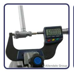
A micrometer can be used to calibrate the bore gauge. Set the micrometer to the desired size and lock. Insert the measuring head between the micrometer.
