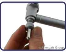
3. Secure with the Collet nut. Do not overtighten.
