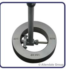
A setting ring can be used to calibrate the bore gauge. Select the desired size setting ring. Insert the measuring head into the measuring ring.
