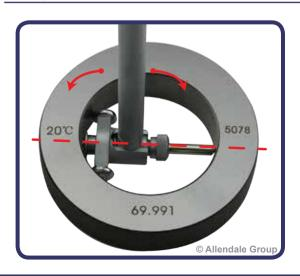
The measuring head centering guides are sprung to help align the measuring contact plunger and anvil contact with the center of the bore when measurements are being taken. Lean the bore gauge at an angle and gently ease into the bore. Gently rock the bore gauge to find minimum reading.
