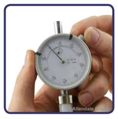
With the gauge inserted parallel between the calibration device, ensure the bezel locking screw is loose. Rotate the outer bezel on the dial gauge to read zero. Tighten the bezel locking screw. The bore gauge is now calibrated.
