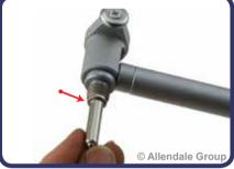
2. Insert the anvil and spacer (if required). These spacers should be placed between the anvil shoulder and measuring head.
