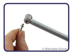
1. The gauge needs to be set with suitable anvils and spacers for the bore being measured. The anvil contact and measuring contact plunger should touch both sides of the bore and compress by approximately half the measuring plunger travel.
